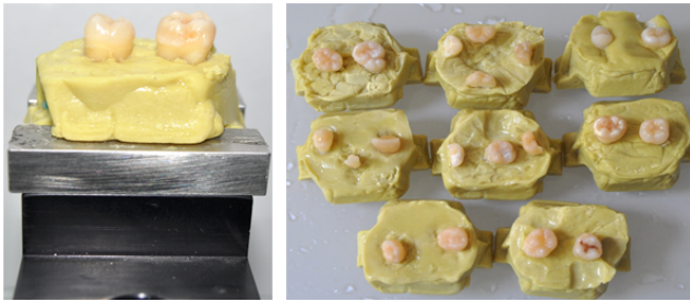
Fig. 2. Teeth fixed acrylic resin and prepared for fixing the ceramic rods on enamel and dentin
